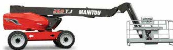
The 260 TJ from Manitou features a working height of 26m
